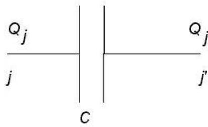
Fig. 3 A capacitor  $C$ .
