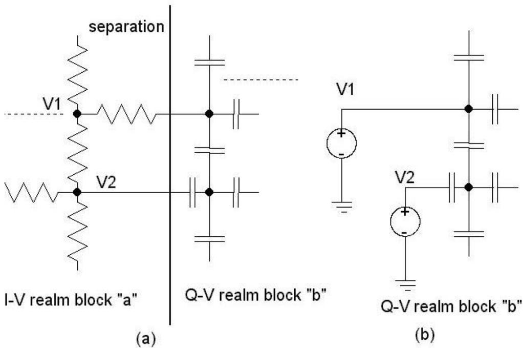
Fig.5 An interface between I-V and Q-V realm blocks.
