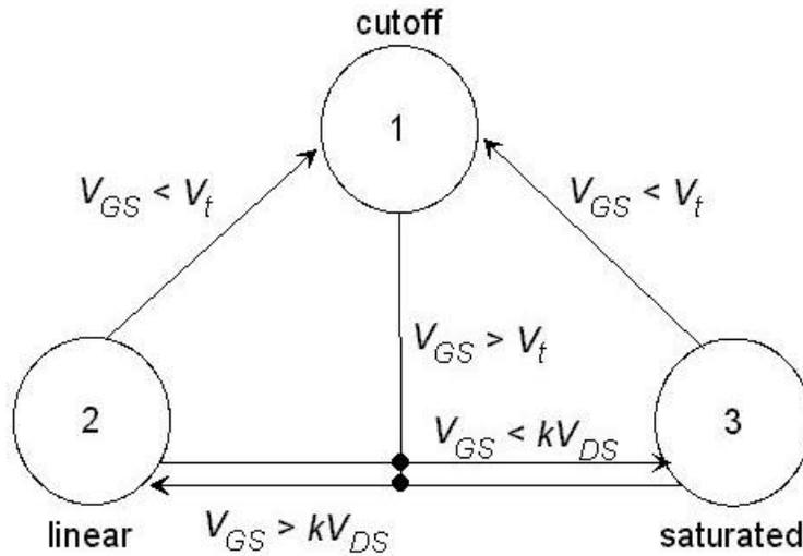
Fig. 2 Dynamic state transition diagram of a MOS transistor.
