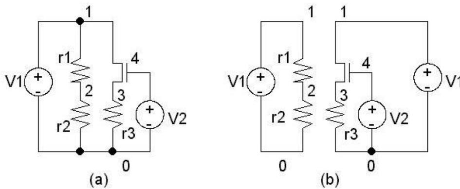
Fig. 4 A node tearing example.
