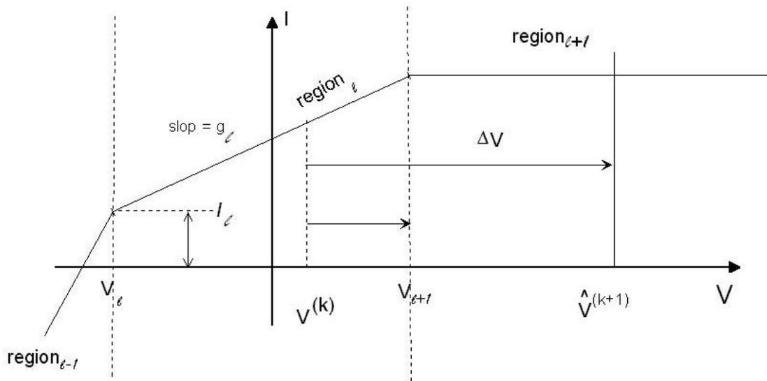
Fig. 1 A voltage controlled resistive device.
